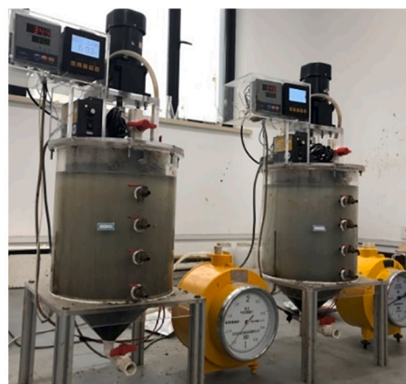
Fig. 1. Schematic of the semi-continuous AD reactors used in this research.
